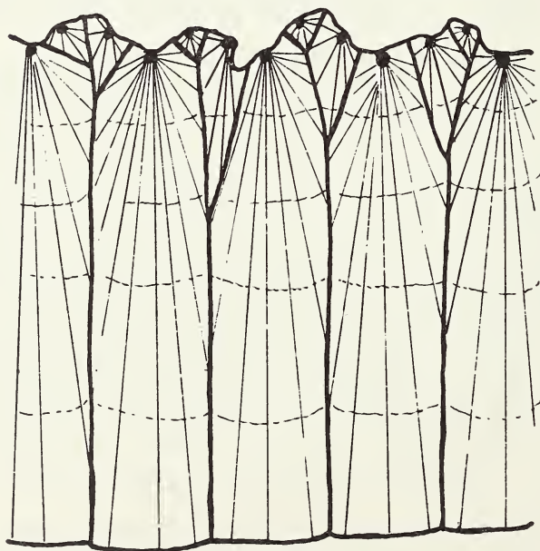
FIGS. 19-21. This series of diagrams, based on spherulitic growth in an inorganic system (Grigor'ev 1965) arising from an irregular surface, shows the internal structure of the spherulites and the development of prismatic structure. The structures are very similar to those seen in the prismatic layers of bivalves. The elimination of some spherulites and the increase in size of the remaining prisms as a result of geometric selection is also comparable to that of the bivalves.
